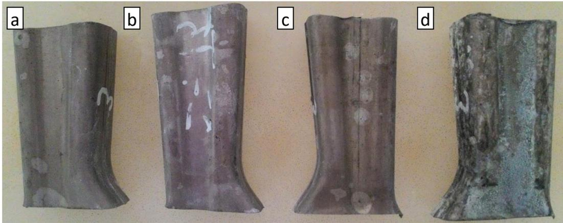
**Figure 4.** Photos of specimens after 21 days (near 500 hours) of salt spray test ST (a) 0.27 (b), 0.45 (c), and 0.89 (d) respectively.
