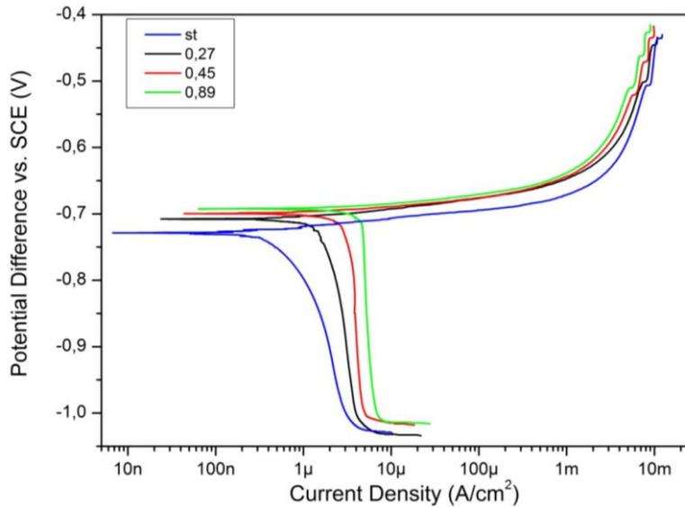
Figure 6. Tafel curves of alloys, between  $\pm 300$  mV.
