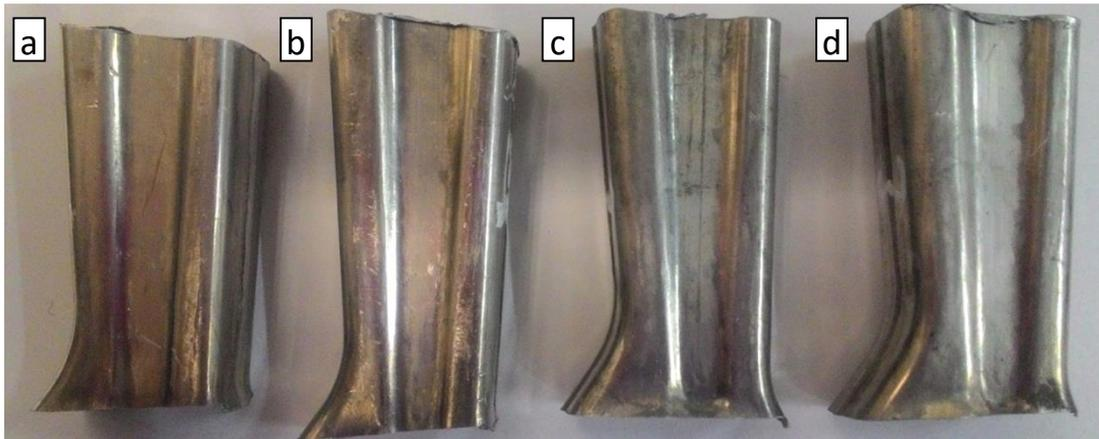
**Figure 3.** Photos of specimens after 15 days (near 350 hours) of salt spray test ST (a) 0.27 (b), 0.45 (c), and 0.89 (d) respectively.
