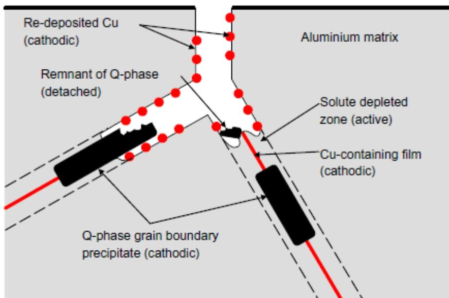
**Figure 1.** IGC mechanism, conceptual (7).
