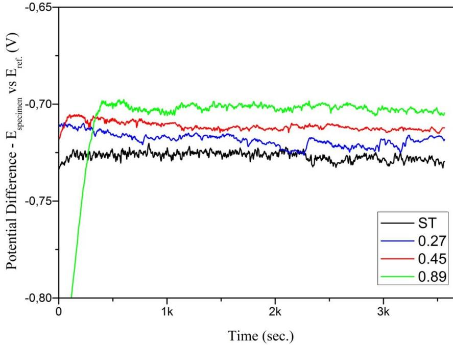
Figure 5. Open circuit potentials of alloys over 1 hour of measurement in 2 wt.% NaCl solution.
