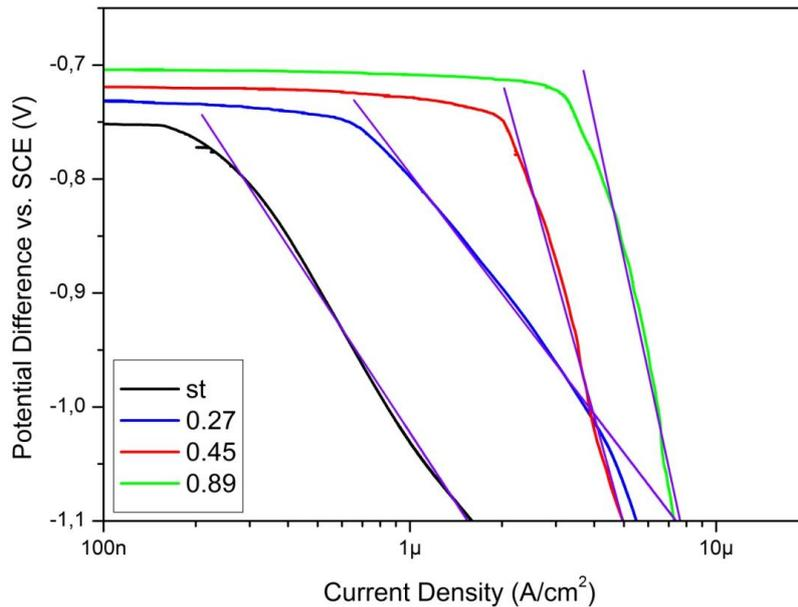
**Figure 7.** Cathodic polarization curves of alloys with linear fit.
