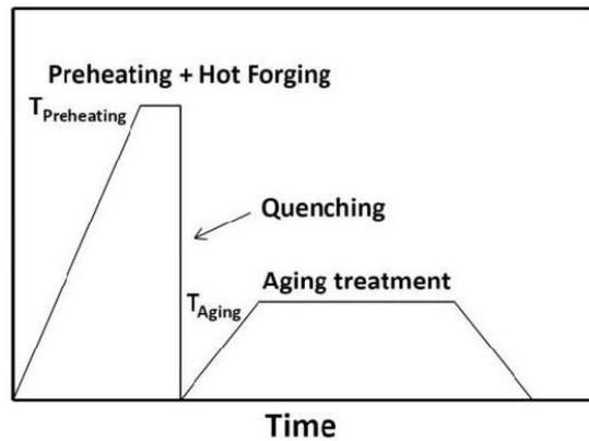
**Figure 2.** T5 processing of extruded bars.
